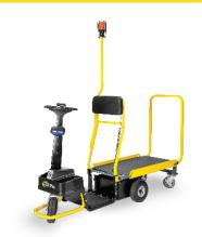
Deck size: 40" x 22" 1,100 lbs. overall capacity 42.5" turn radius 81" L x 26" W x 62" H
